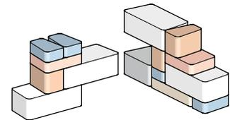
Place block in an overlapping, interlocking pattern at corner for added wall stability.
