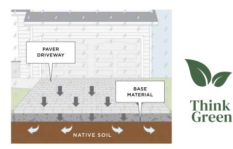
Developed in response to growing concerns around stormwater management, permeable pavers allow rainwater to flow between the joints and back into the subsoil. This provides a dual "green" benefit: it reduces the amount of water sent to storm sewers, and instead provides extra moisture to surrounding plant material.
